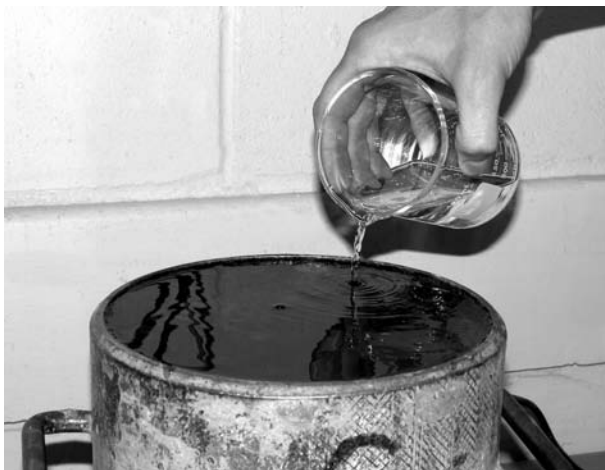
FIGURE 7.6 Calibrating the measure—determining the measure volume. (Photo courtesy of Karol Kowalski and Adam Rudy, Purdue University.)
