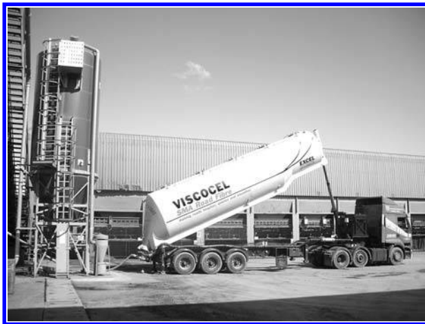
FIGURE 4.9 Tractor-storage bin unit loaded with granulated stabilizer. (Photo courtesy of Excel Industries Ltd., U.K.)
