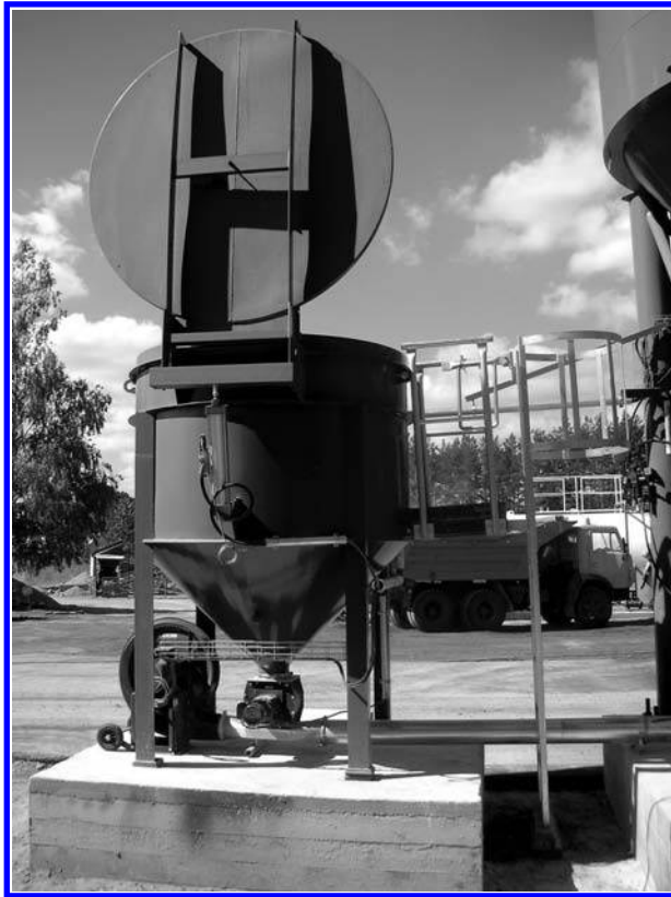
FIGURE 9.7 A system for batching granulated fibers into mixing plants. The photograph shows an open silo for granulates ready for loading. (Photo courtesy of Bartosz Wojczakowski.)
