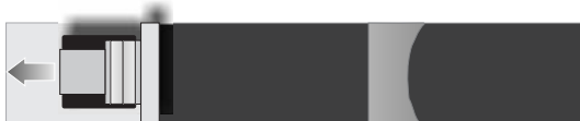
FIGURE 11.15 Area of an uncompacted cool mixture during a paver standstill (a zone of cooling mixture that is inaccessible to rollers).
