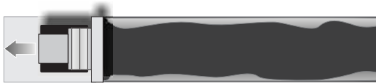
FIGURE 11.19 Manually corrected edges of a working lane with cooler temperatures and higher porosity.
