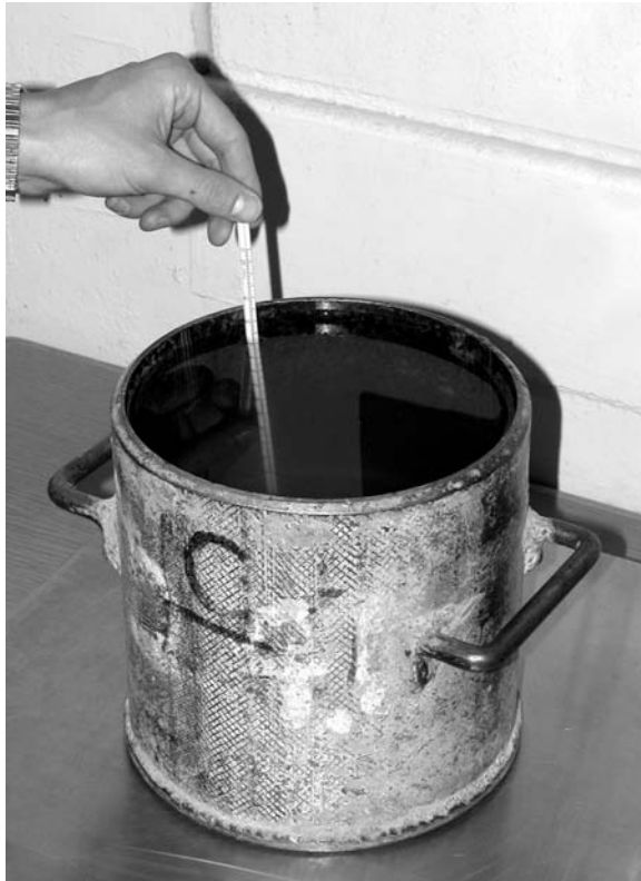
FIGURE 7.5 Calibrating the measure—determining the water temperature. (Photo courtesy of Karol Kowalski and Adam Rudy, Purdue University.)
