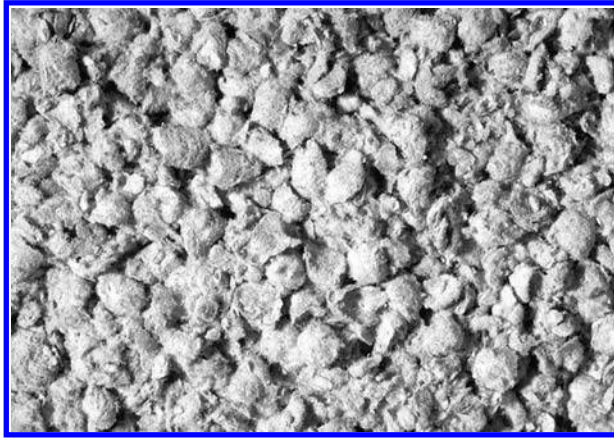
FIGURE 4.5 An example of pellets—loose formed fibers. (Photo courtesy of J. Rettenmaier & Söhne GmbH + Co. KG, Germany.)
