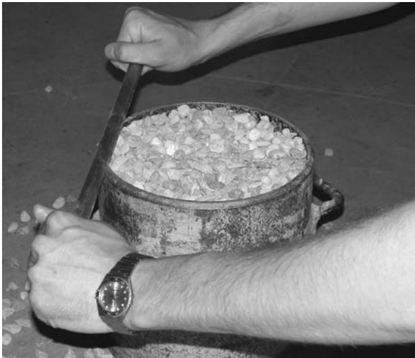
FIGURE 7.8 Clearing away the excess aggregate. (Photo courtesy of Karol Kowalski and Adam Rudy, Purdue University.)
