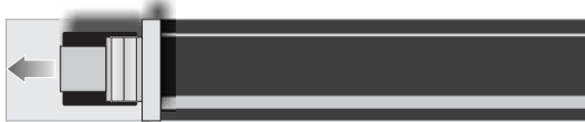
FIGURE 11.13 Formation of streaks or mixture pulling due to incorrect setup of paver screed segments.
