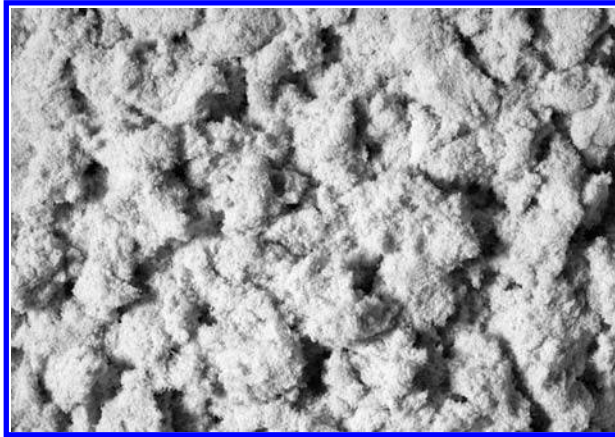
FIGURE 4.4 An example of loose cellulose fibers. (Photo courtesy of J. Rettenmaier & Söhne GmbH + Co. KG, Germany.)
